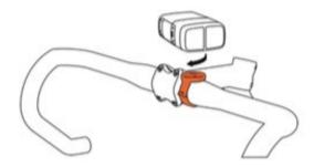
2. With your Fly12 facing forward, and at a 45° angle, line up the quick release male component on the Fly12 with the female receptor on the handlebar mount. Place the Fly12 into the mount and make a 1/8<sup>th</sup> turn until the device clicks into a forward-facing position. The distinctive 'click' sound confirms the unit has been locked in place.
